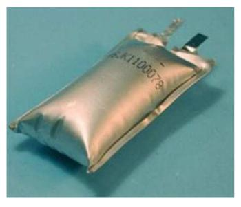
The result of the overcharge is damage to the cells.
